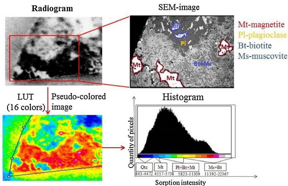
**Figure 2** Steps of the technique of relative sorption efficiency definition. Combined analyses of radiogram of Ra sorption on the 166 sample and the corresponding SEM image of the same fragment of 166 sample.
